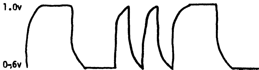
Output of LM3900 op-amp during record. Goes to tape recorder.
