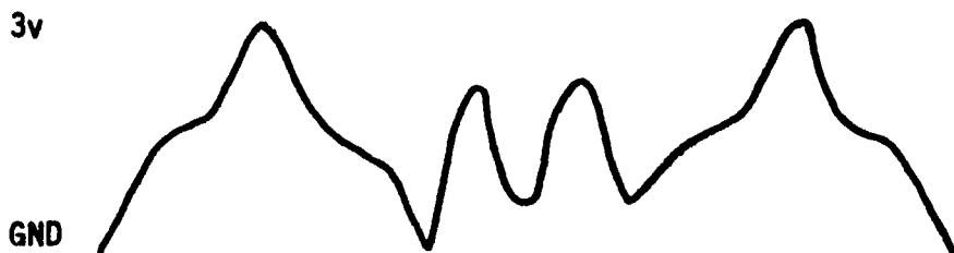
Output of tape recorder on playback. Elf squares it back up to original shape with a LM3900 & sends it to EF2.
