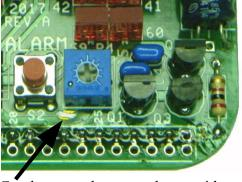
( ) Cut the trace shown on the top side of the board to disconnect VCC from the collector of Q2.
