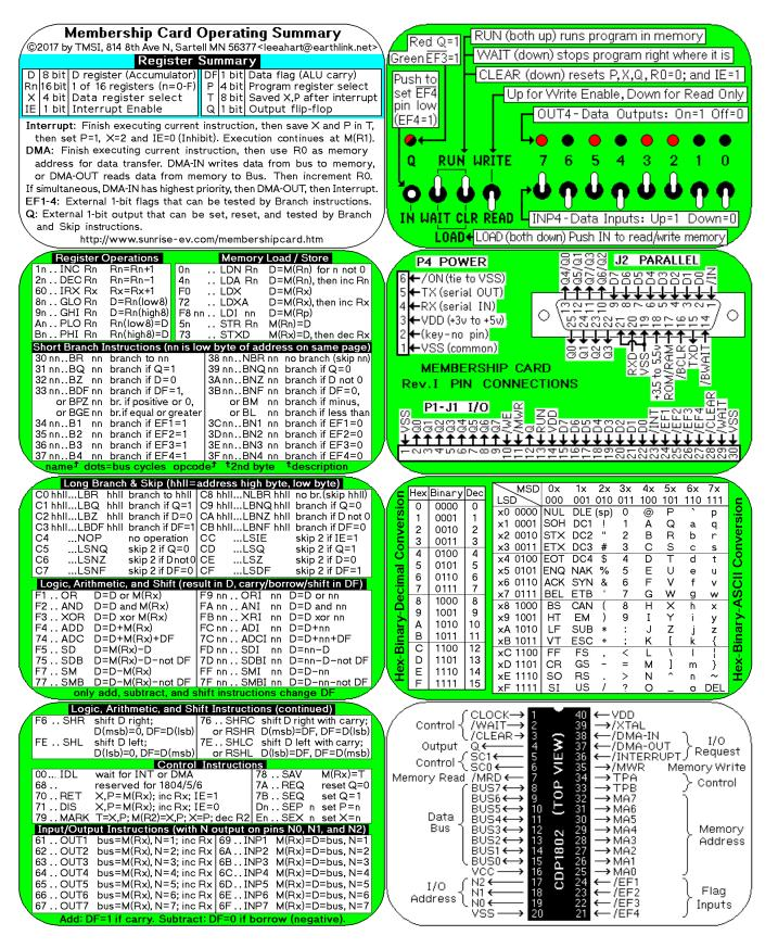
Membership Card Summary: Keep the left half in the manual, in case you need to make a copy later. Cut the right half out, fold, and put in the Altoids case as a quick reference (& so board won't short to case).
