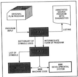
3. Compiler. Translating PL/M programs into machine language takes two passes with programs called PLM1 and PLM2, run by a larger machine. A third pass, with Interp/8, simulates the microprocessor on the big machine to check out the program.
