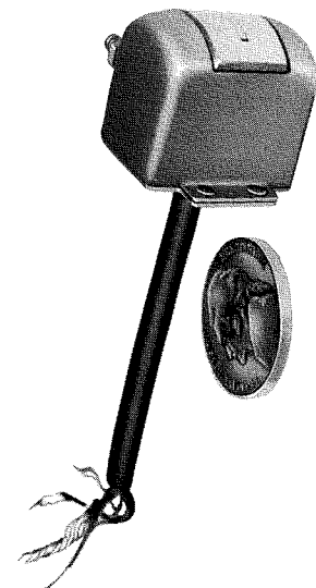
Fig. 3—Finished stereo head in shielded case.
