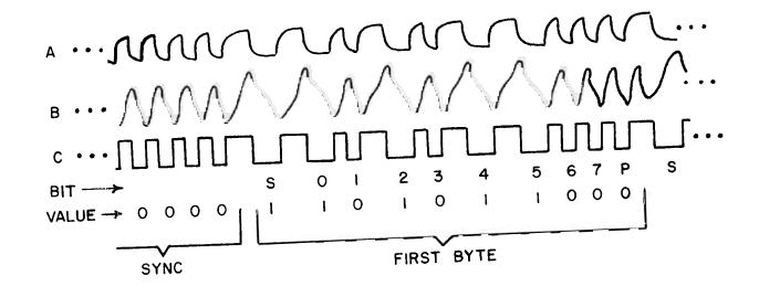
A-OUTPUT OF UI4A B-OUTPUT FROM CASSETTE (TAP IN PAD ON CARD) C-OUTPUT OF UI4B
