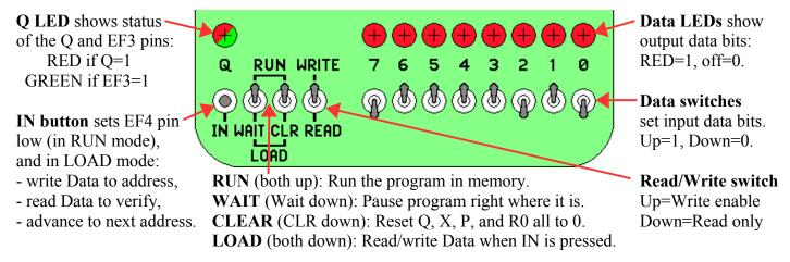
Let's load a program and see if it works! For each step, set the switches as shown. "1" means the switch is up. "0" means the switch is down. "X" means push and release the IN button. "." means the switch position doesn't matter. I'll show the switch positions like this:
